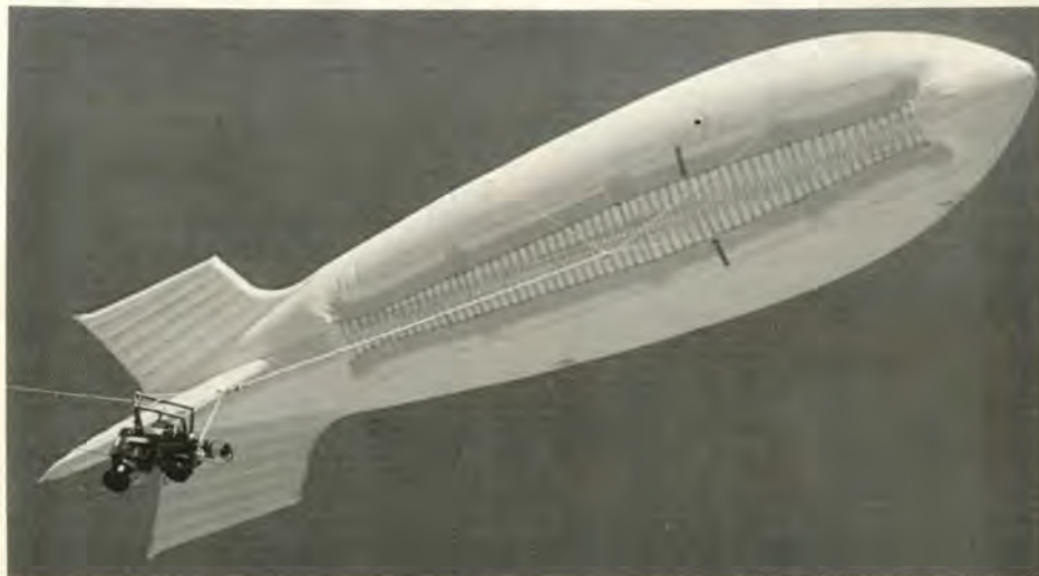
The ten-meter blimp lifts its twin cameras for vertical site recording.
