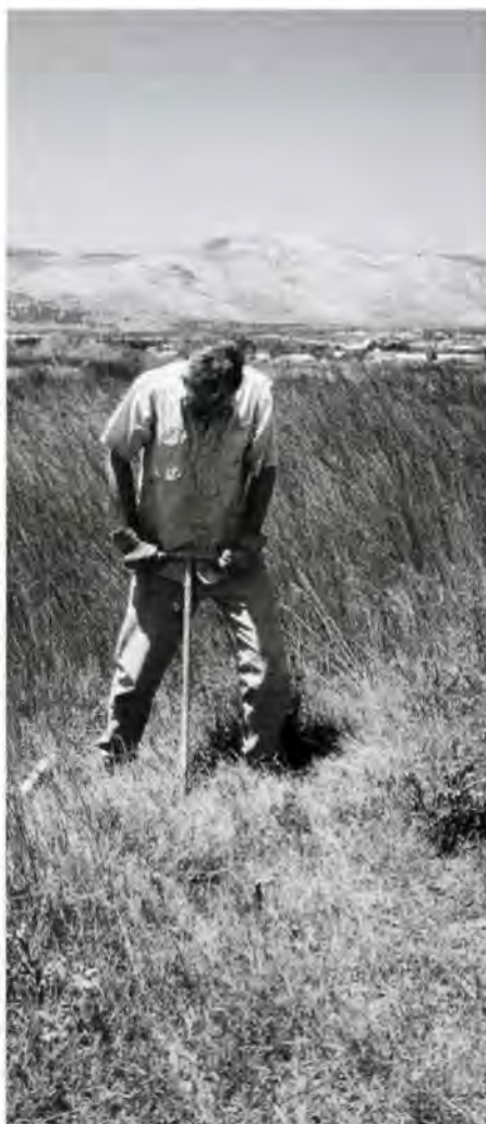
Richard K. Dunn takes hand-driven auger core sample from Marathon Plain.
