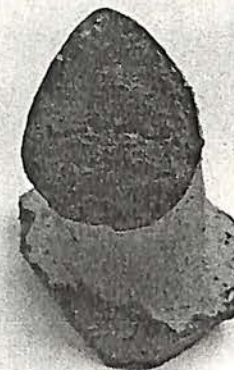
Fig. 20. Cross section of a fourth-century handle showing cracking and random alignment of inclusions. Formation of the handle was thus by rolling rather than pulling. Since the handle is the thickest part of the jar, the radial cracking shown here is quite common (C-1978-79).
