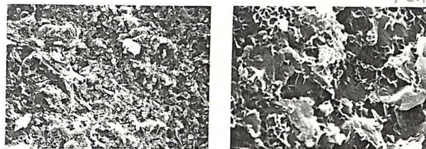
Fig. 35. Scanning electron microscopy micrographs taken at x 1000 (left) and x 10 000 (right) of fracture surfaces showing the vitreous microstructure of a Corinthian A gray core (same sample as shown in Fig. 4).
